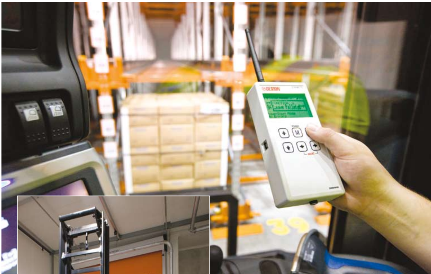
Shuttle controls have been integrated into the truck itself for operator efficiency and ease
